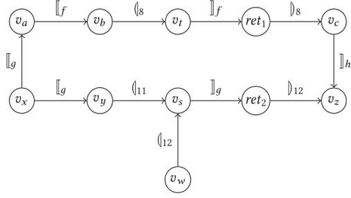
(b) INTERDYCK-reachability graph for taint analysis. Bracket edges (i.e.,  $\llbracket_f$  and  $\rrbracket_f$ ) represent field reads and writes w.r.t. a field name  $f$ . Parenthesis edges (i.e.,  $\langle_l$  and  $\rangle_l$ ) represent calls and returns w.r.t. the line number  $l$  of the call-sites.
